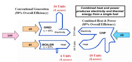
Energy efficiency advantage of a cogeneration system (UNESCAP, 2000)
