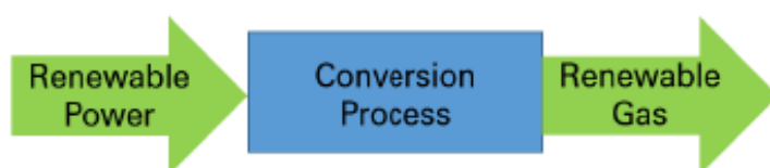
Figure 2: Simplified Power-to-Gas process (AGFW, 2019)
