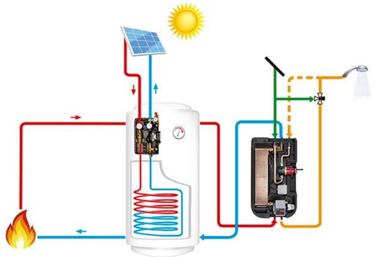
Figure 14: Diagram of fresh water station and tank. Source: Orkli [12]
